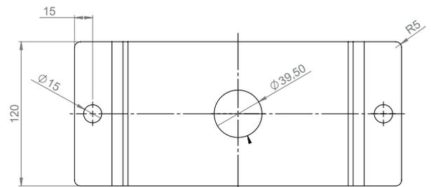
Dimensioning of ceiling bearing for grating, for square caps or lockable attachment
