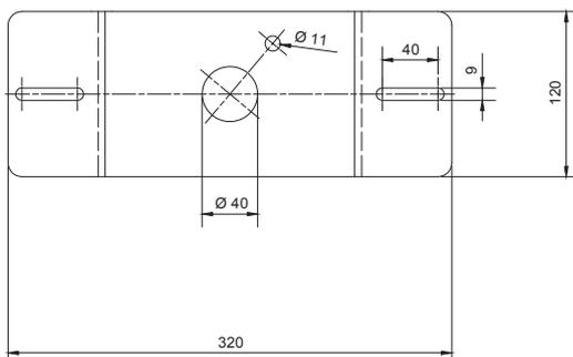
Dimensions of ceiling bearing for grating for position indicator
