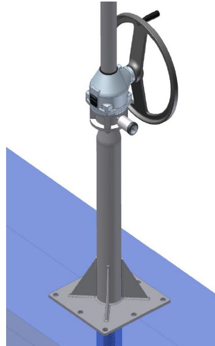
Grease-cartridge at the bearing of a penstock with rising spindle
