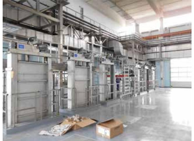
12 XL3 channel penstocks 3-side sealing 1200 x 6650 mm as two-spindle version
