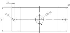
Dimensioning of ceiling bearing for grating, for square caps or lockable attachment
