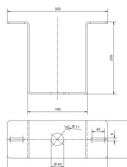
Dimensions of ceiling bearing for grating for position indicator
