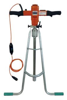
MOBITORQ electric with drive rod, end position damper and drive stand
